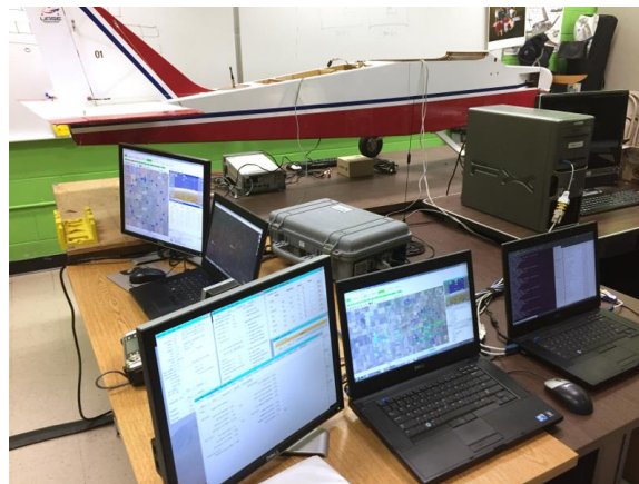
Figure 57. Full simulation testbed; GPC 1, bottom; GPC 2, right; GPC 3, upper left; external flight systems and GCS, top.
