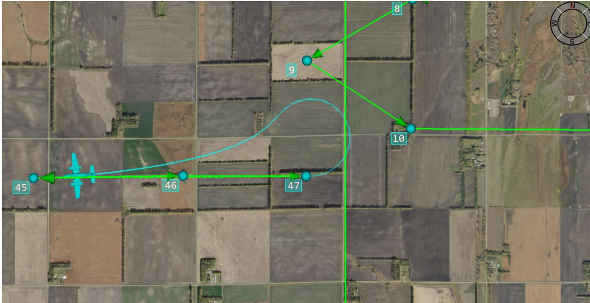
Figure 67. Emblematic crop-duster maneuver: climbing P-Turn to reverse course. Apex of turn beyond waypoint 48 crosses ownship path (N-S in green) at or near same altitude as ownship.
