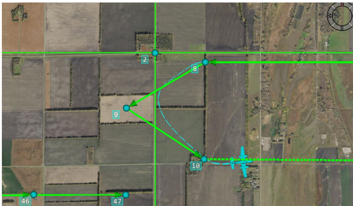
Figure 66. Emblematic crop-duster maneuver: climbing U-Turn to reverse course. Apex of turn (short of waypoint 9 when configured for pre-turn logic) approaches ownship path (N-S in green) at or near same altitude as ownship.
