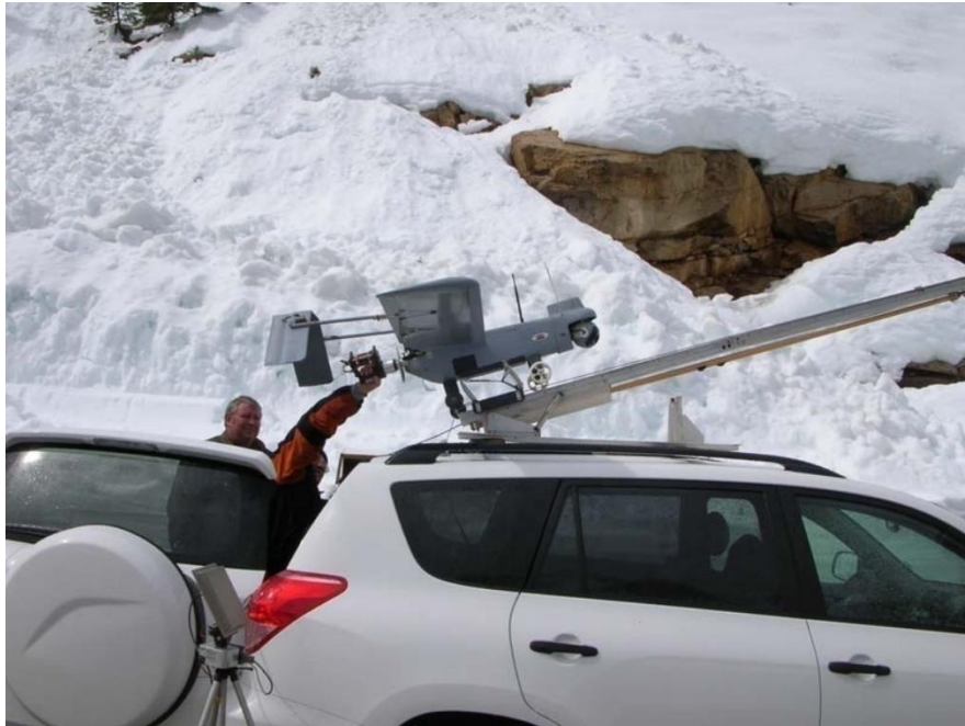
Figure 21. MLB BAT platform catapult launch (McCormack, 2008).
