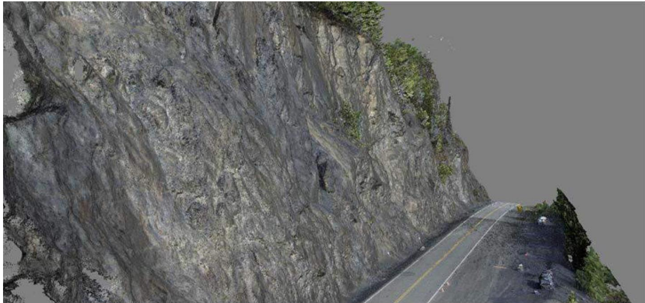
Figure 19. 3D model of rock slope generated from UAS imagery (Cunningham et al., 2016).
