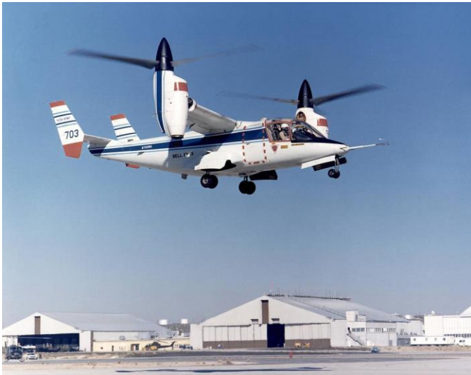
Figure 3.81 Bell XV-15 tiltrotor in hover (NASA, 1980).
