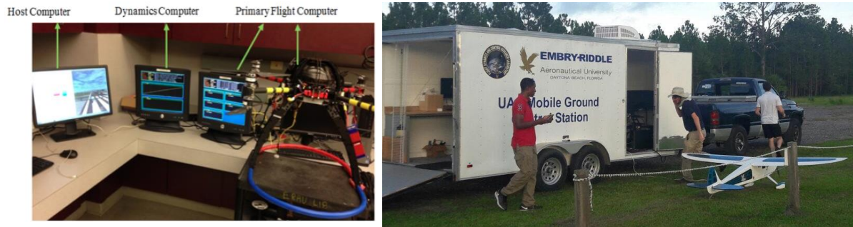
Figure 8. (a) Hardware-in-the-Loop UAS Simulation Platform; (b) Mobile Ground Control Station for UAS.
