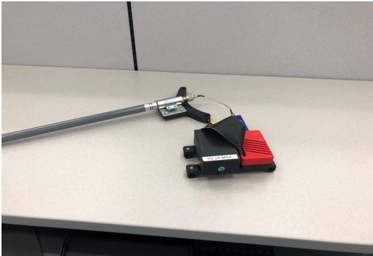
Figure 1. ADSB Logger Payload tah was integrated into an Aurelia X6 hexacopter.
