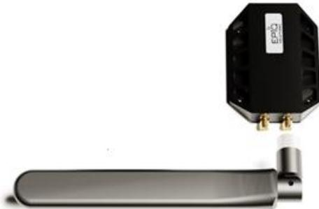
Figure 19. Prism scanner is the black unit with the antenna (detached).
