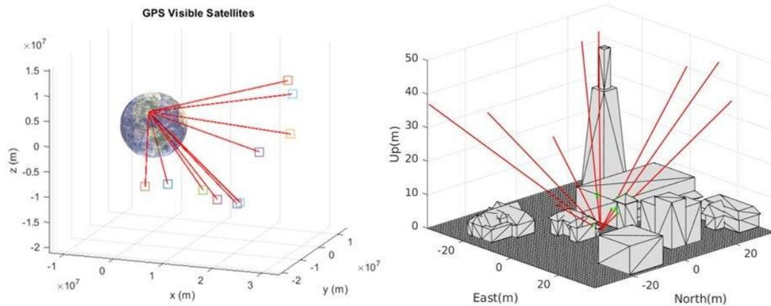
Figure 47. GNSS Signal Modeling for Shadowing Multipath Effects.
