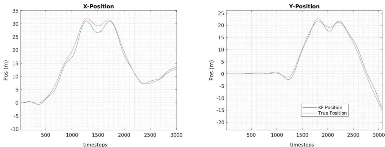
Figure 70. Position Estimation integrating OF Velocity Measurements.
