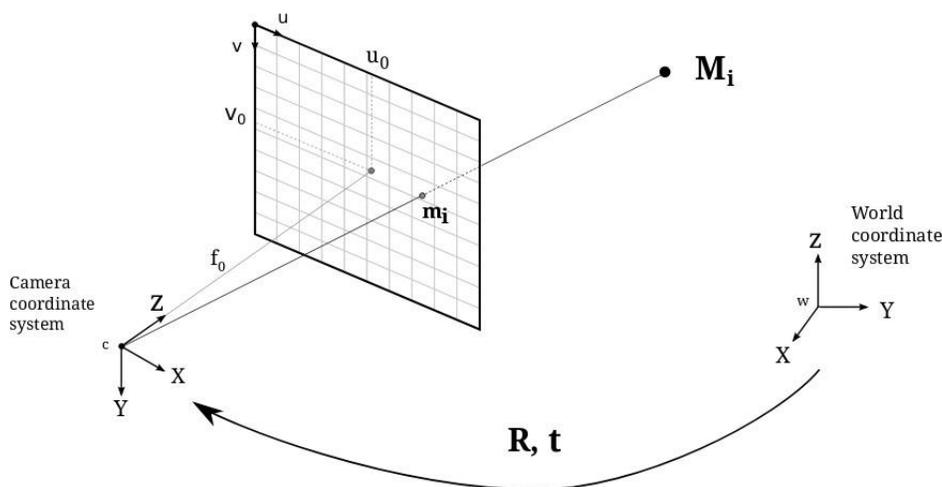
Figure 55. Pinhole Camera Model.
