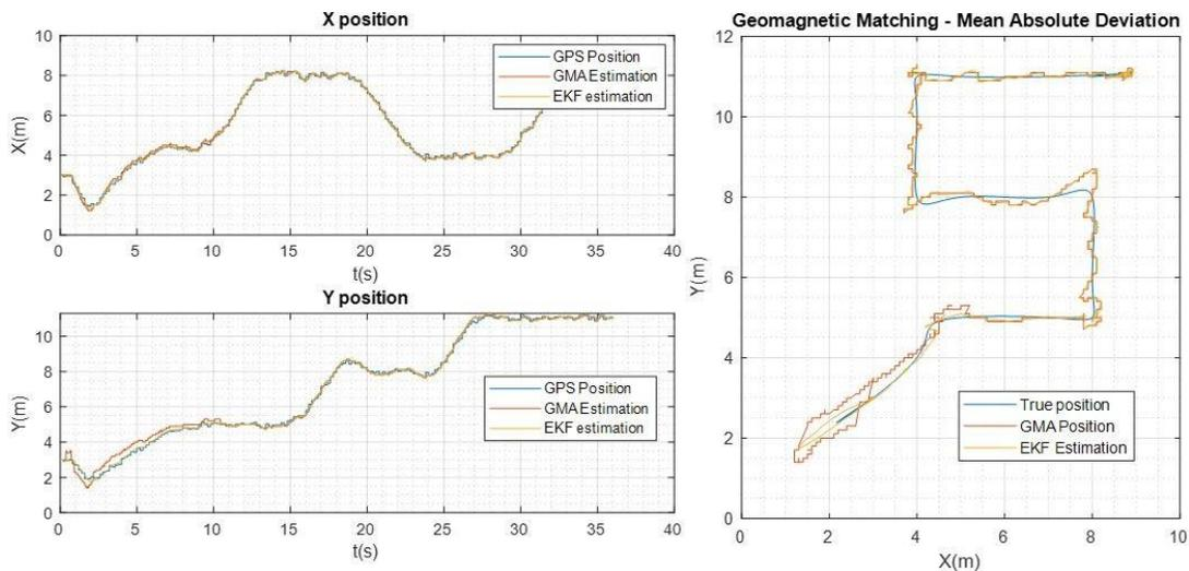
Figure 75. Trajectory S - Geomagnetic Matching Position estimation.
