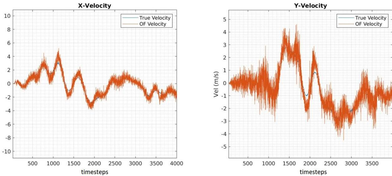
Figure 68. Velocity Measurements by only Optical Flow Odometry.
