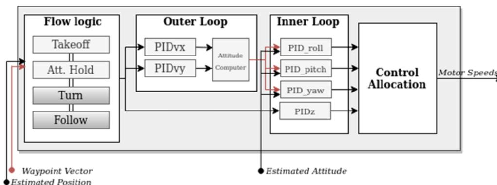
Figure 52. Position Control Scheme with Fuzzy velocity referencing.
