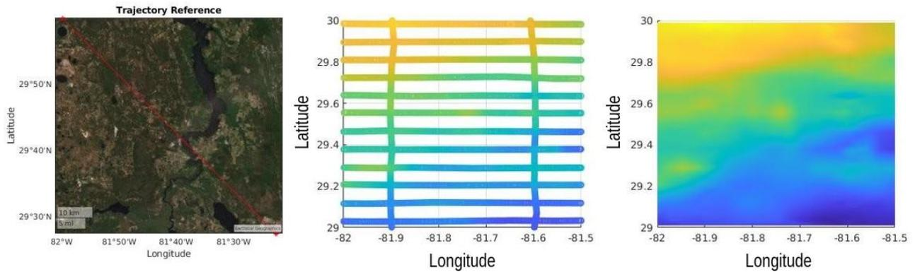
Figure 58. Anomaly magnetic mapping by extensive aerial measurements.
