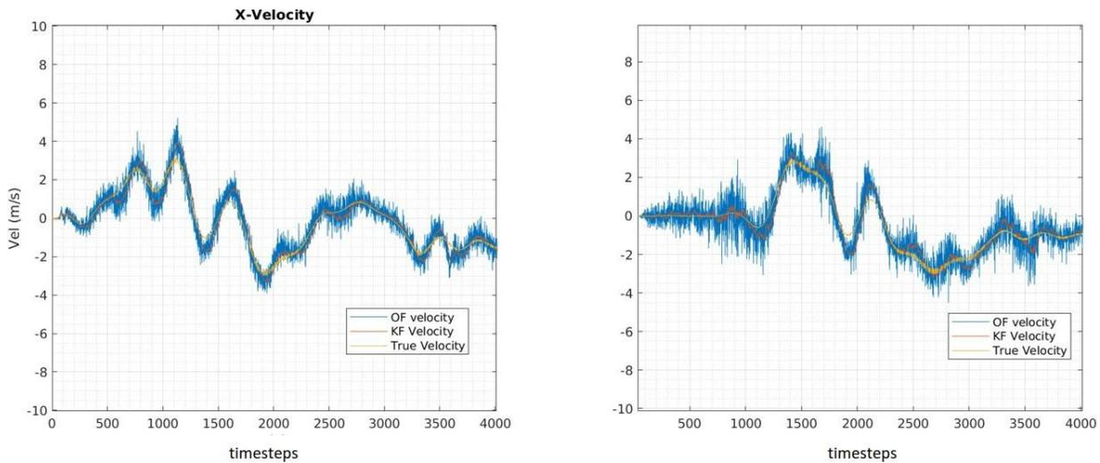
Figure 69. Velocity Estimation integrating OF Velocity Measurements.
