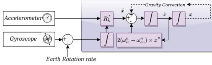
Figure 51. Inertial Mechanization.
