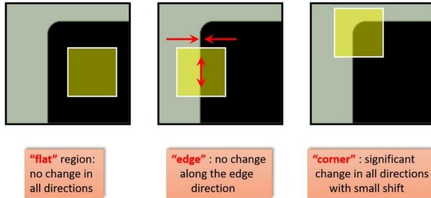
Figure 54. Illustration of Intensity use for Corner and Edge Detection (G. Bradski 2000).
