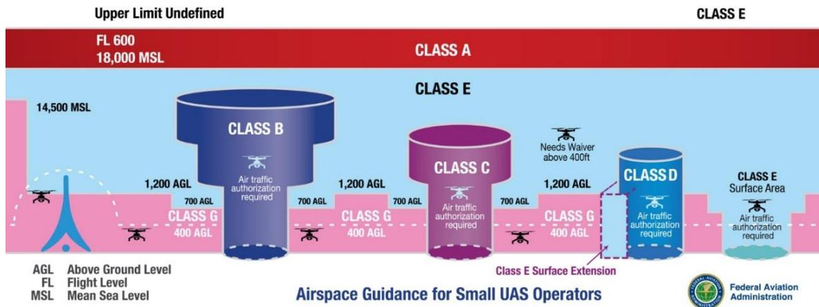
Figure 9. FAA specified operating altitudes for UAVs based on classes (Federal Aviation Administration 2018).
