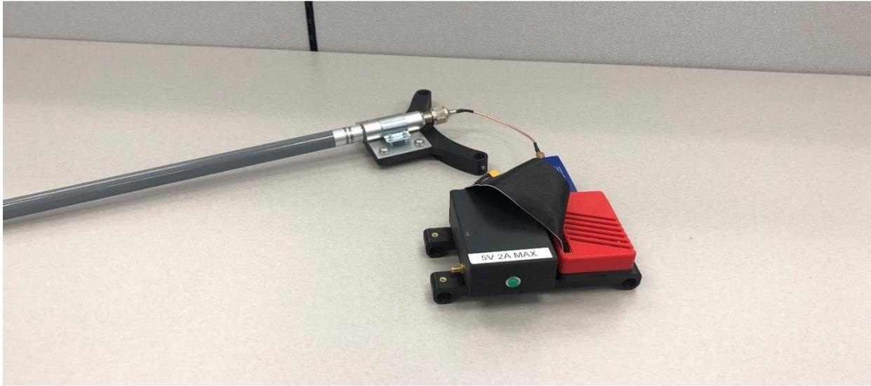
Figure 12. ADS-B Logger Payload.
