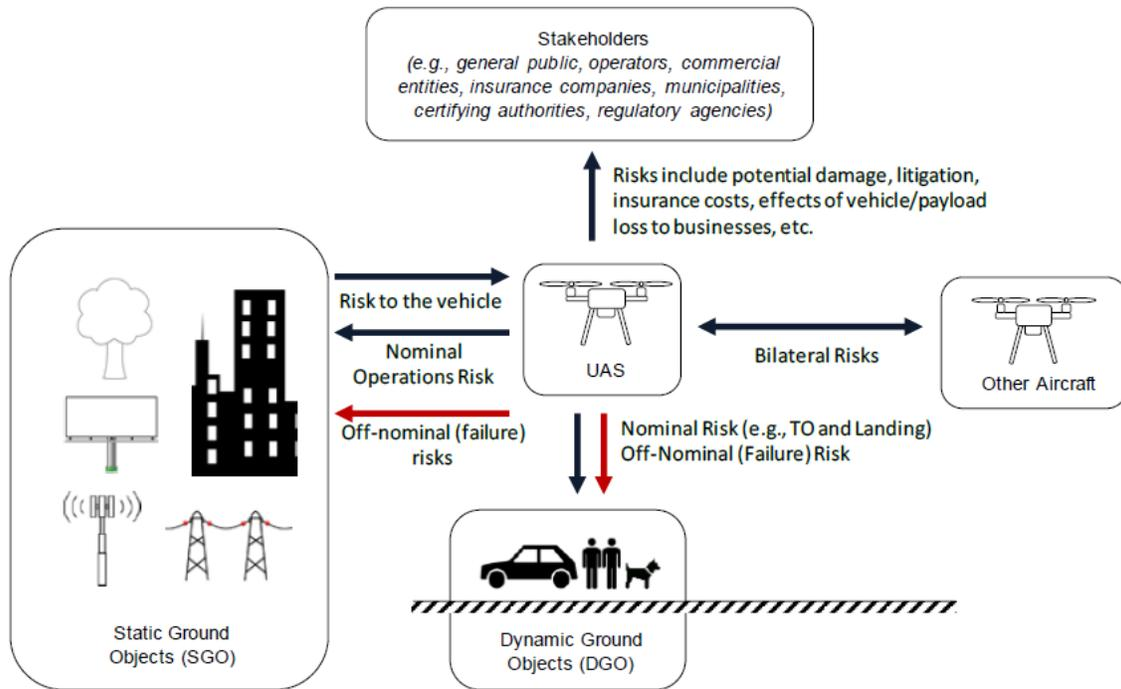
Figure 16. UAS Vehicle-Centric Risks and Hazards (Ippolito et al., 2019) – SAFE50 reference design study for large-scale high-density low-altitude UAS operations in urban areas.
