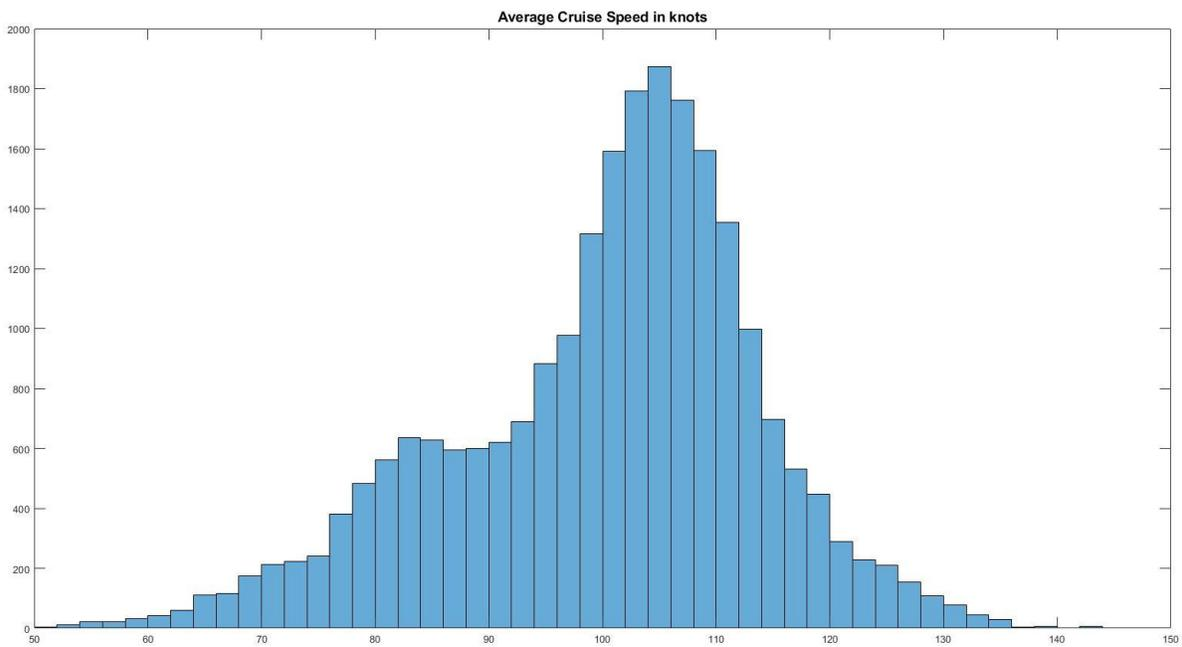
Figure 7. Average cruise speed distribution (kts), with number of files on the vertical axis (Raspet Flight Research Laboratory, 2020)
