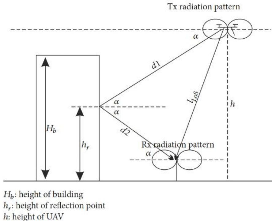
Figure 14. Sketch of the reflection from the sidewall (Qiu, 2017)
