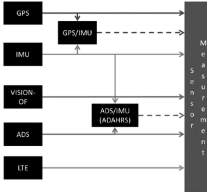
Figure 15. Sensor System Diagram (Rufa & Atkins, 2016).
