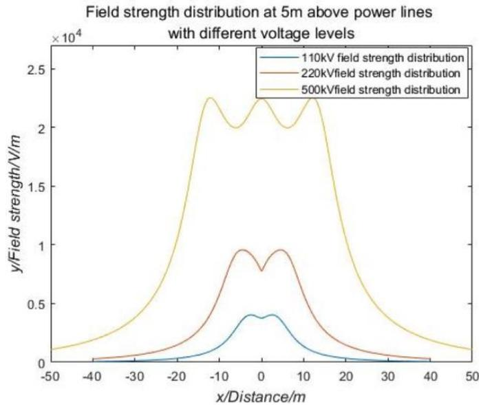
Figure 13. Distribution of field strength at 5m above transmission lines for different voltage levels (Heggo et al. 2019)
