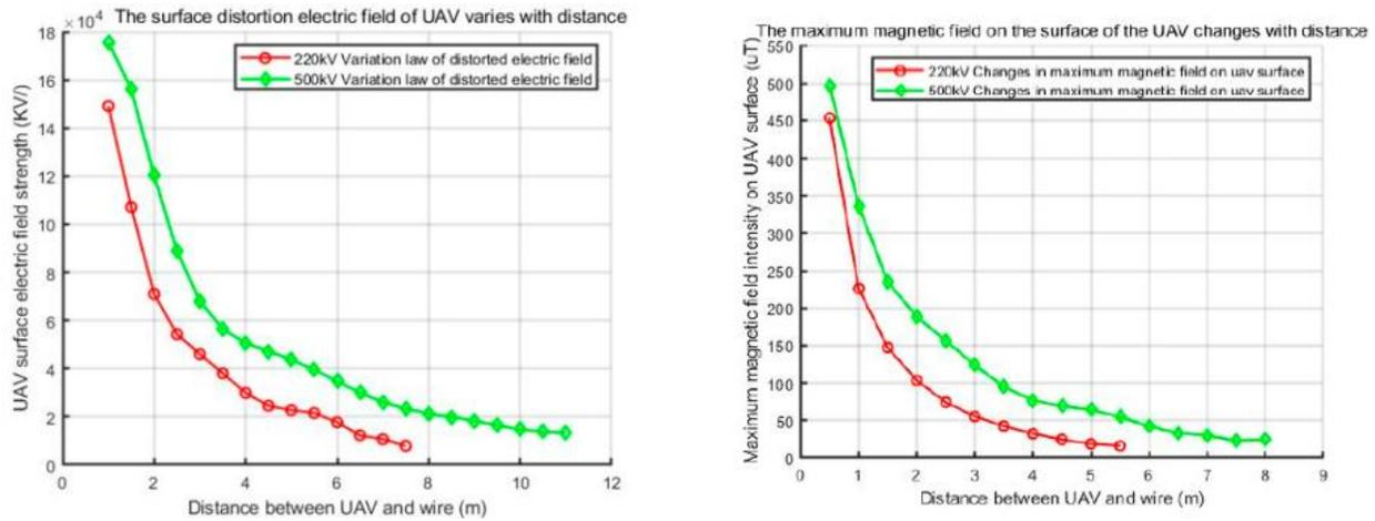
Figure 12. Variation of surface distortion electric field of UAV with distance and Maximum magnetic field on the surface of the UAV changes with distance
