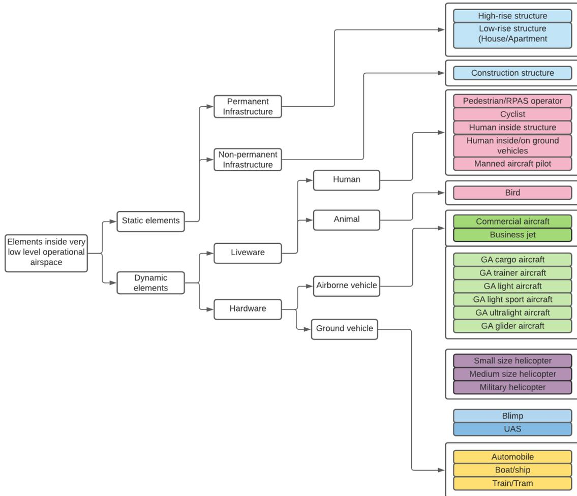
Figure 9. Object classification flowchart, both ground and airborne objects (modified from: RattanaGraikanakorn et al., 2018).
