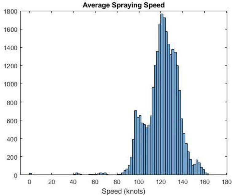
Figure 5. Spraying speeds, with number of files on the vertical axis (Raspet Flight Research Laboratory, 2020)
