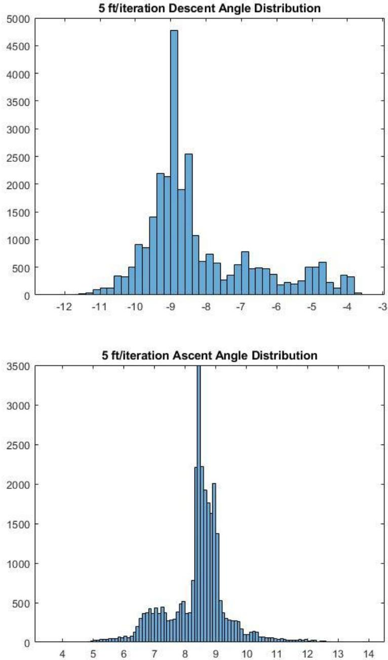
Figure 3. Aircraft trajectory angles relative to the Earth's surface for descent-into (top) and ascent-from (bottom) spraying runs. Number of files are on the vertical axes (Raspet Flight Research Laboratory, 2020).
