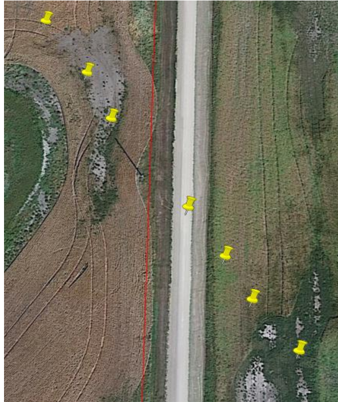
Figure 10. Example of an aircraft interaction with a powerline. The yellow pins show aircraft locations and the red line indicates the powerline.
