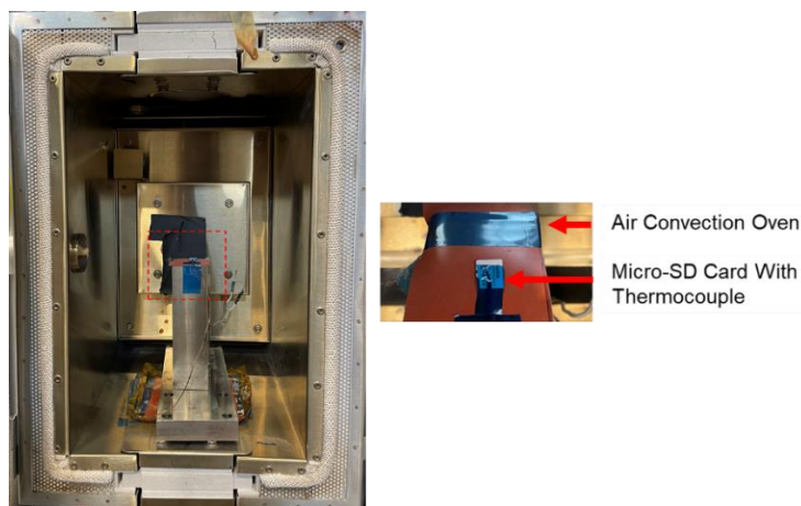
Figure 5. Low-intensity fire test setup.
