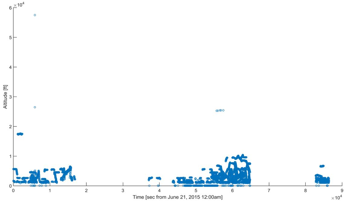
**Figure 6.5. Altitude [ft] vs. time [sec from June 21, 2015 12:00a.m.] plot showing aircraft w/ the same aircraft ID number. There were many readings that occurred at the same time period, indicating that multiple planes had the same ID number.**
