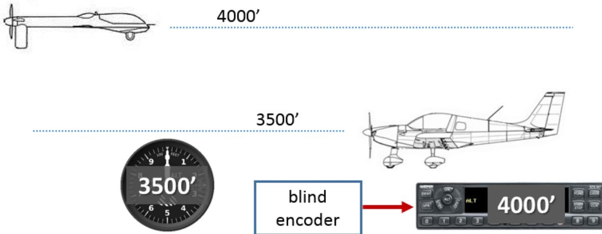
Hazard 7 examines the conflict between a DAA-equipped UAS and a no-transponder aircraft intruder where the intruder has a static system error – flight instruments reports an altitude different from the actual aircraft altitude. Depending on the aircraft altitude and distance from an ATCRBS site and the installed ADS-B ground network, two aircraft in close proximity in this hazard can take on the four subcases detailed above.
