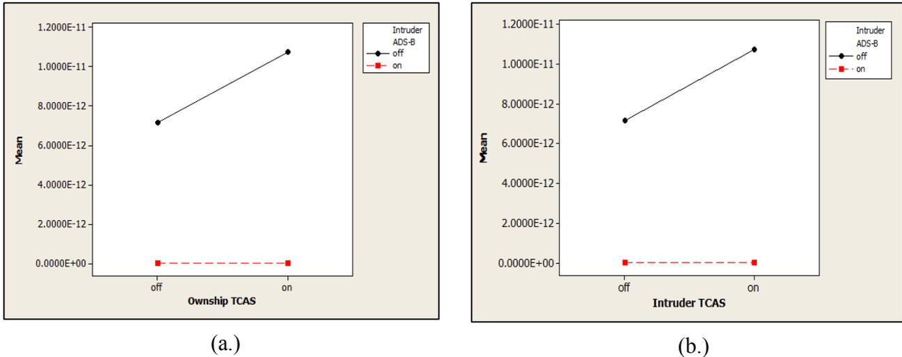
**Figure 6.3. Interaction plots depicting how total likelihood varies simultaneously depending on two factors: Ownship TCAS and Intruder ADS-B (a) and Intruder TCAS and Intruder ADS-B (b). In both cases, while intruder ADS-B (red dashed line) is on, failure likelihood doesn't change when TCAS turned on, but in the case of Intruder ADS-B off (black solid line), likelihood increases when TCAS turned on.**
