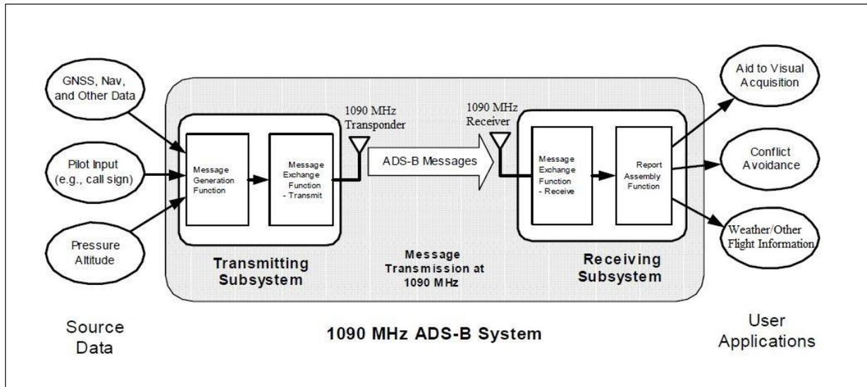
**Figure 3.1. ADS-B block diagram**
