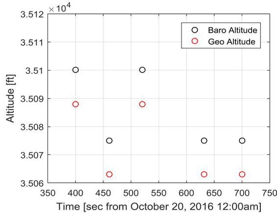
**Figure 6.10. Altitude [ft] vs Time [sec from October 20, 2016 12:00am] plot showing cyclic change in both geometric and barometric altitude data**
