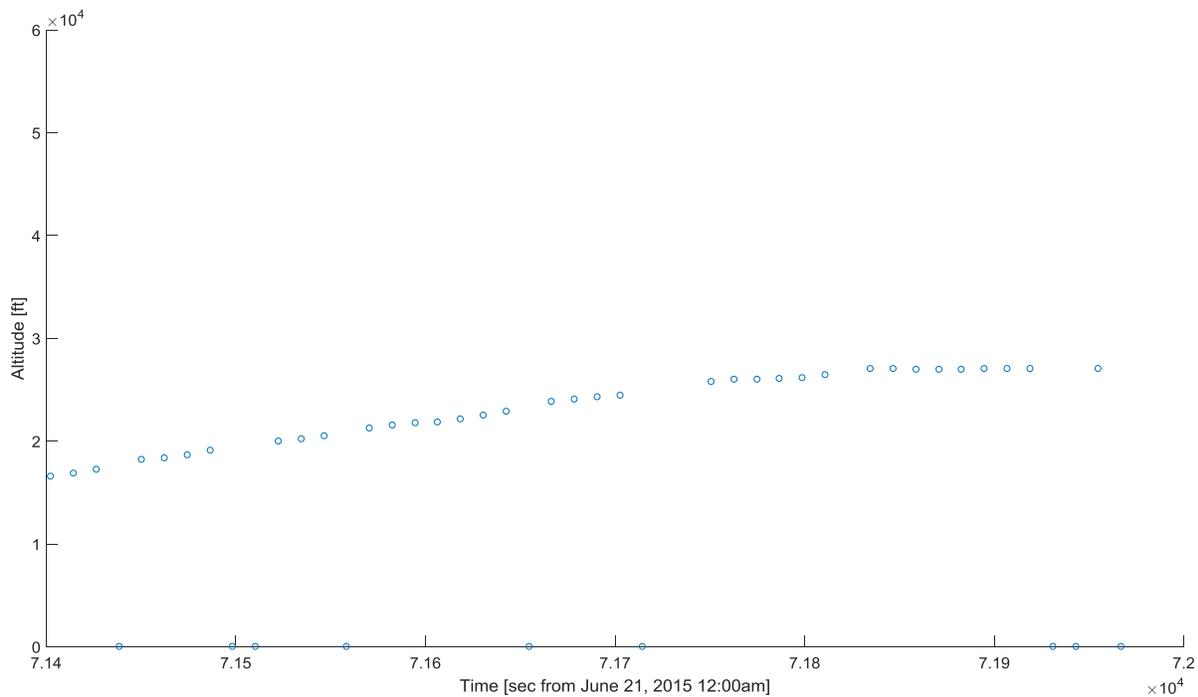
**Figure 6.6. Altitude [ft] vs. time [sec from June 21, 2015 12:00a.m.] plot showing outliers. Note how the altitude readings jump from their nominal reading to 0ft back to the nominal value many times.**
