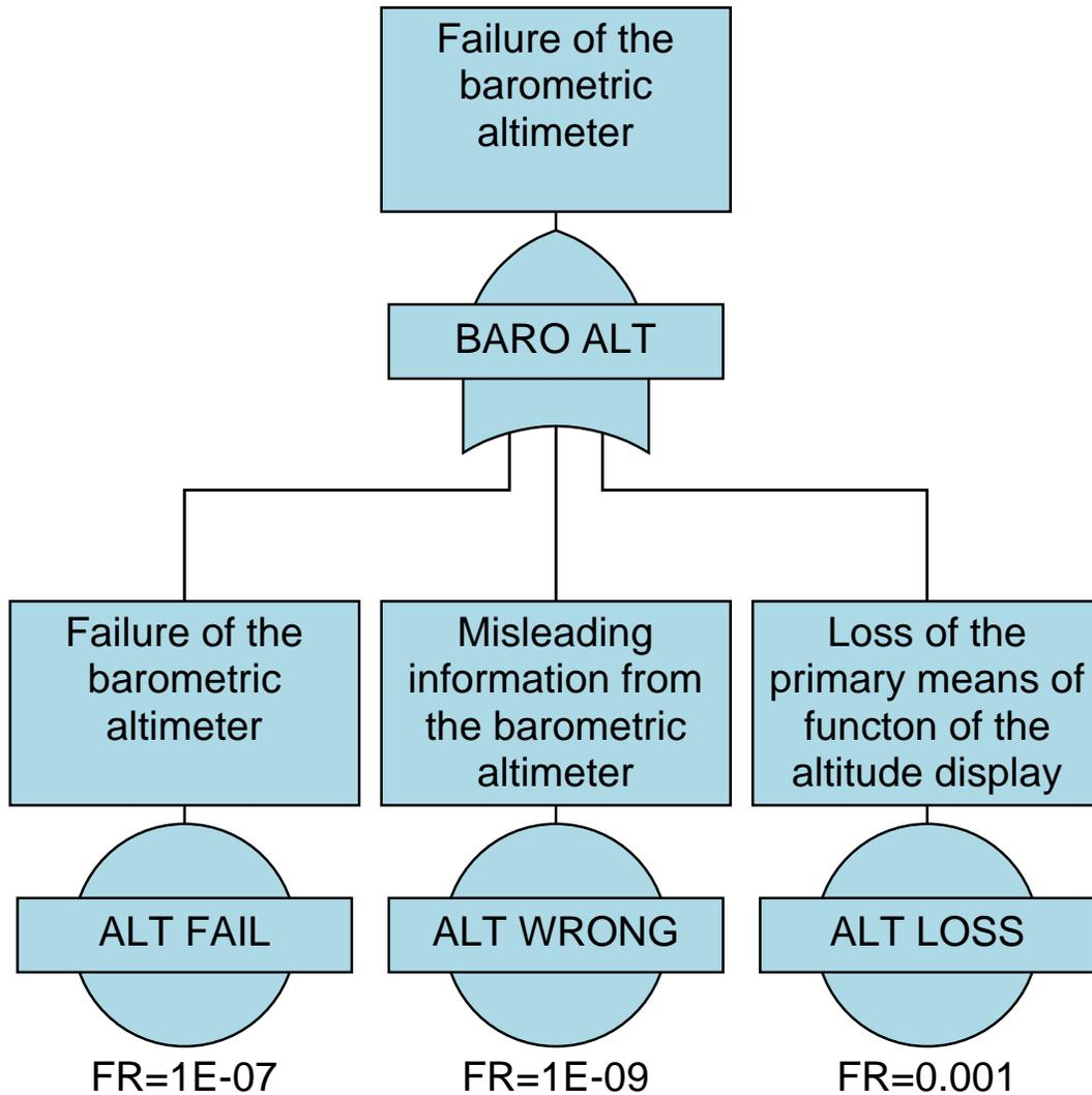
**Figure 5. 10. Barometer altimeter failure tree**
