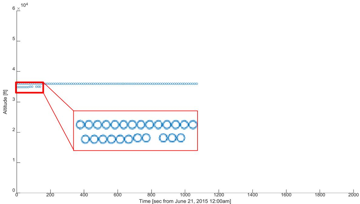
**Figure 6.4. Altitude [ft] vs. time [sec from June 21, 2015 12:00a.m.] plot showing cyclical unique behavior. Note the zoomed in view in the red box showing the altitude reading jumping between two relative values.**
