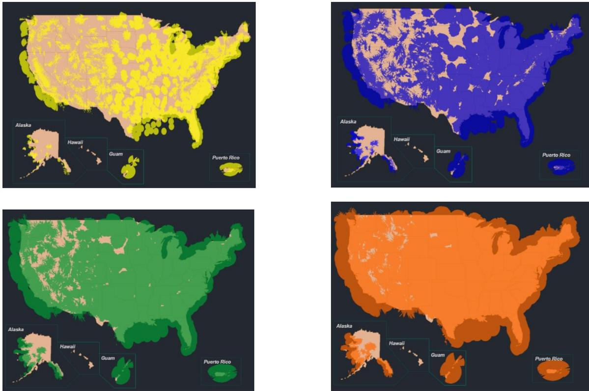
**Figure 10.1. ADS-B ground station network coverage at 500 feet (upper-left), 1500 feet (upper-right), 3000 feet (lower-left), and 5000 feet (lower-right). All altitudes are AGL.**
