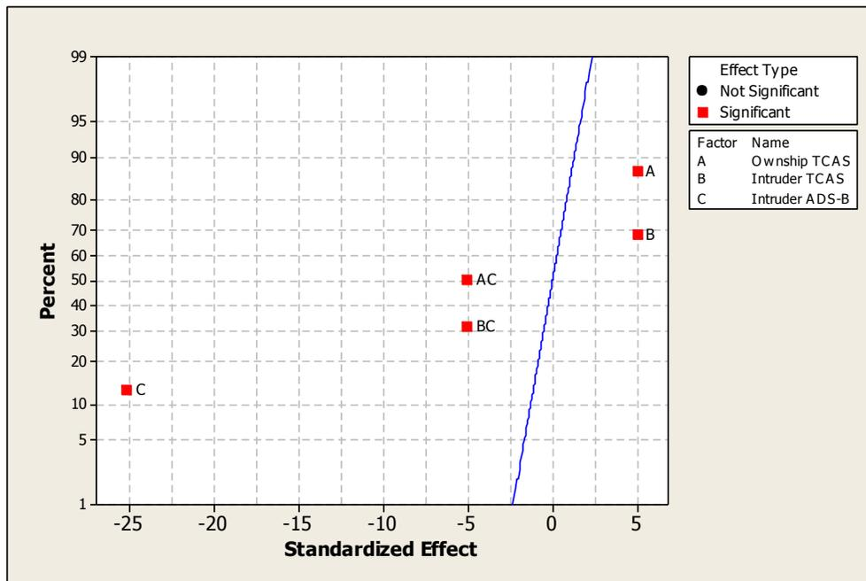
**Figure 6.1. Normal Plot of standardized effects showing factors that had a significant effect on likelihood. The horizontal axis represents the significance of the factor and the vertical axis represents the percentile of the cumulative probability distribution.**
