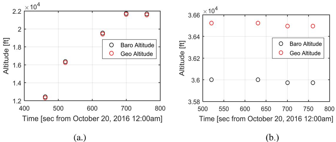
**Figure 6.9. Altitude [ft] vs time [sec from October 20, 2016 12:00am] plots showing discrepancies in ascending and level flight: (a.) Altitude discrepancy is small in ascending phase, (b.) Discrepancy range is higher in level flight.**
