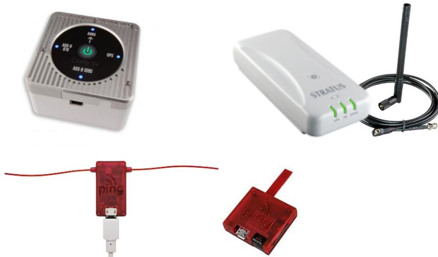
All devices except the Stratus 2 used the device's fixed antenna. The Stratus used an external antenna. The test was a ground based test. The devices were placed within a 1 square foot area approximately 7 feet off the ground. The test was performed from 16:55 – 22:15 GMT on 11/13/16 about 5 miles west of Washington Dulles International Airport (KIAD) in Virginia.
