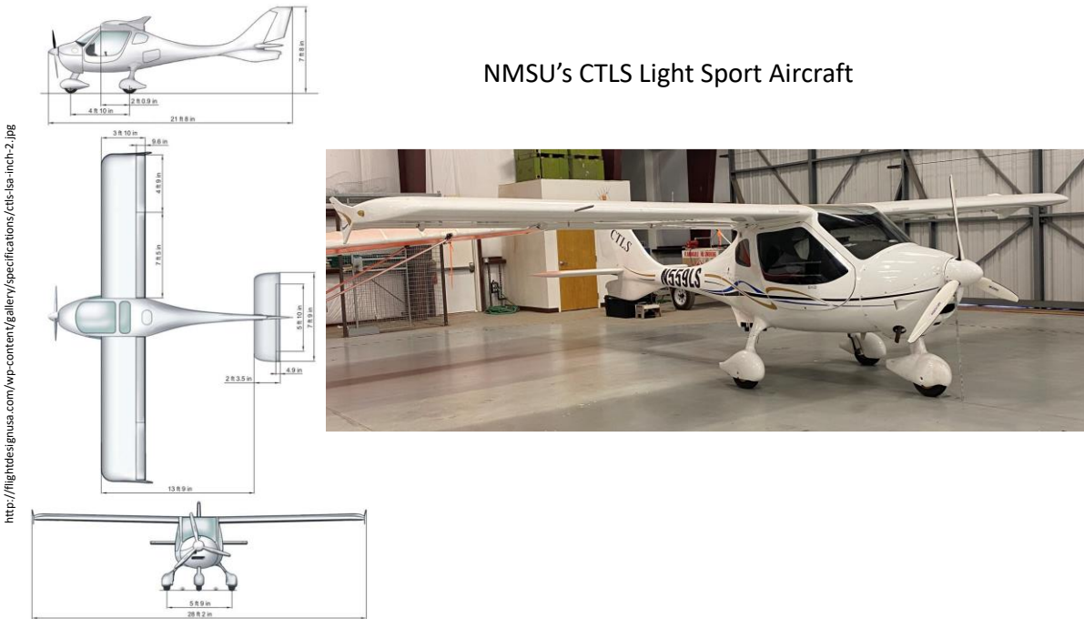
Figure 1. NMSU's CTLS Light Sport Aircraft pictures used for Projected Area Assessment.
