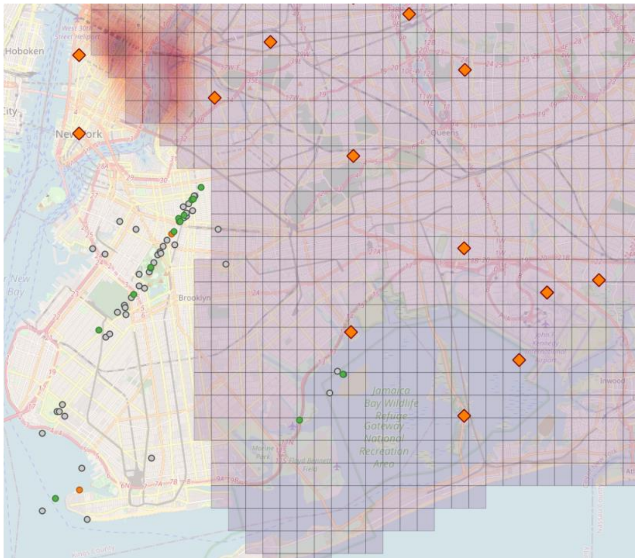
Figure 82. UAS Detection Hotspots with Estimated UAS Sighting Report Locations & Aircraft-UAS Encounters, New York City, NY (Jul 2021-Jan 2022).
