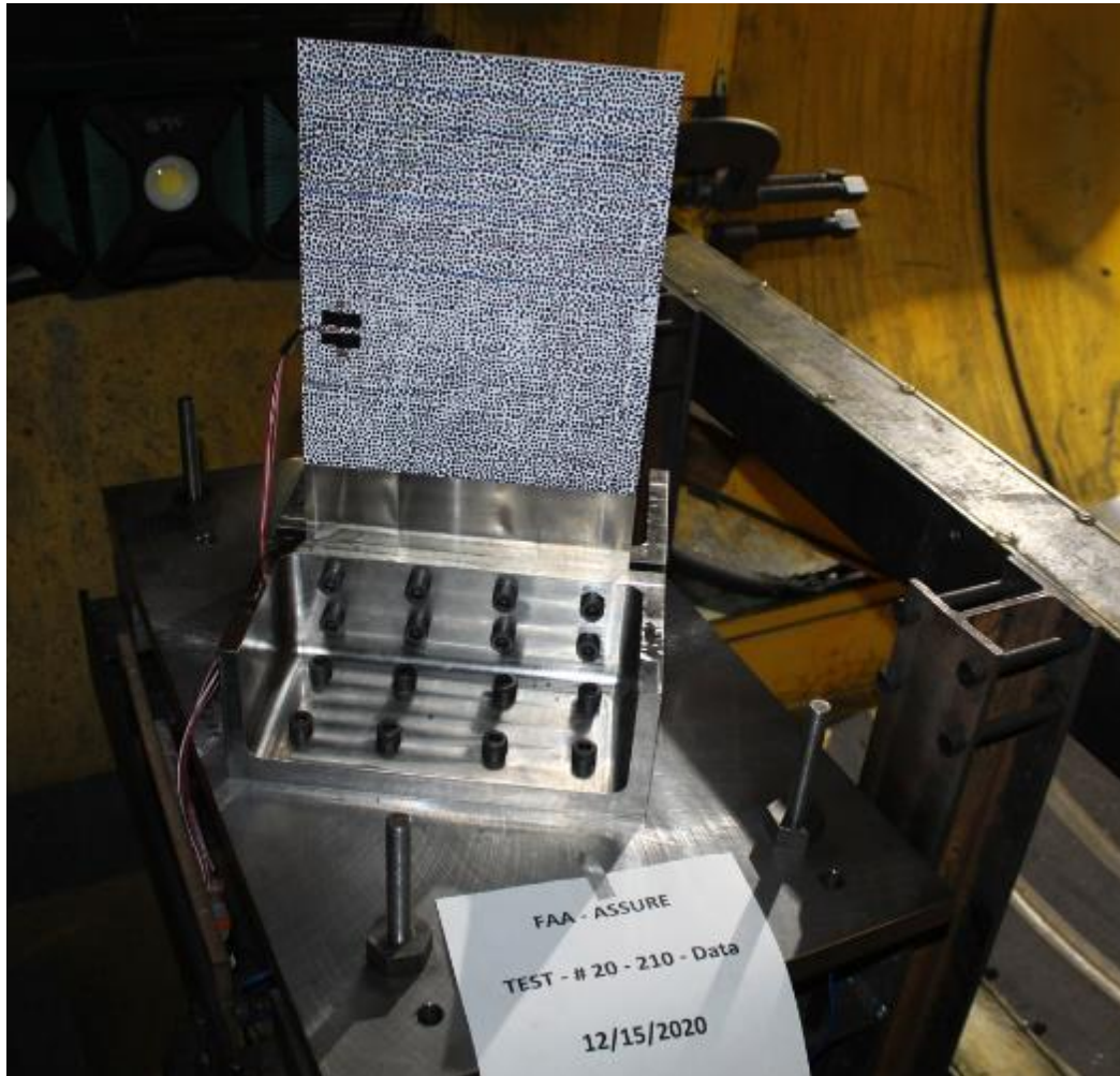
Figure 4. Task A17 Titanium Blade Target, Stainless Steel Bracket, and Tabletop Mount
