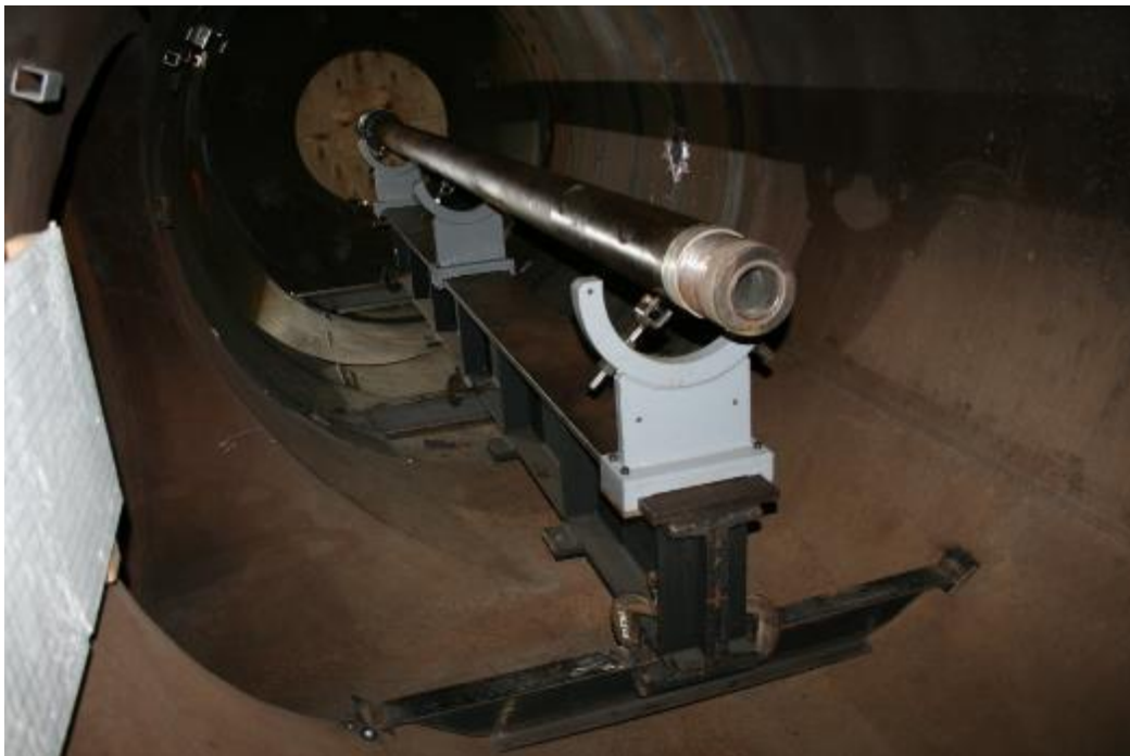
Figure 3. Barrel Extension with Supporting I-beam Structure and Alignment System
