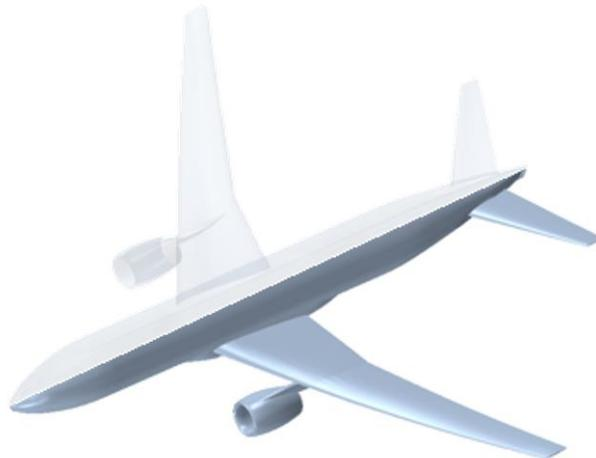
Figure 10. Computational models of the CRM aircraft.
