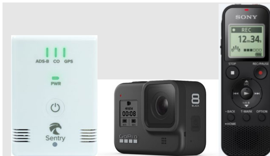
Figure 3. Sentry ADS-B receiver, GoPro Hero 8 Black camera, and Sony PX-470 digital audio recorder used throughout testing.
