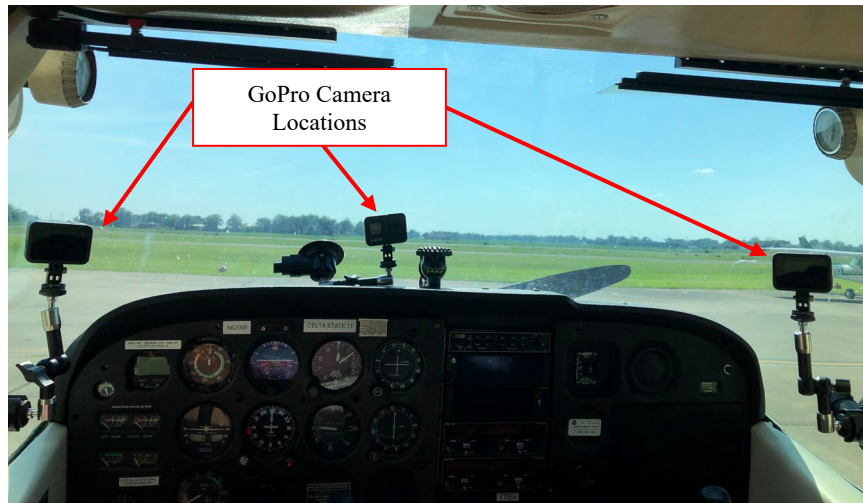
Figure 2. Camera mounting locations in the cockpit of a Cessna 172.
