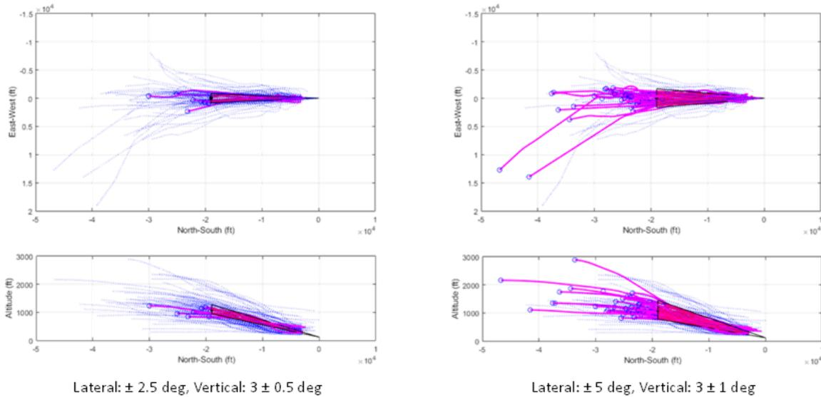
Figure 35. Subset of ownship trajectories meeting the missed approach threshold requirements, shown in pink. Blue tracks do not intersect the approach corridor and were discarded.
