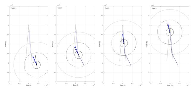
Figure 41. Flight trajectory in chronological order (left to right) of ownship-only case.
