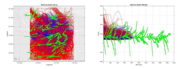
Figure 32. High density clutter. In these charts, ownship trajectories are shown in blue, intruders in red, and clutter in green.
