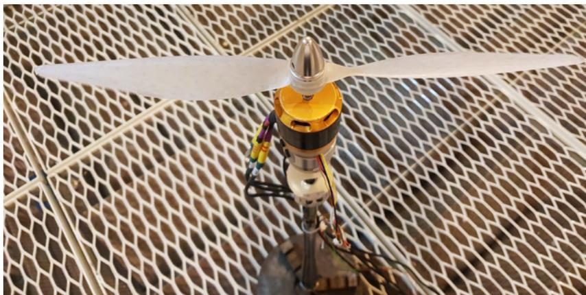
Figure 2.1: Propeller rig in the anechoic chamber. The encoder is positioned below the motor shaft and the ATI Mini40 load sensor is placed under the encoder.
