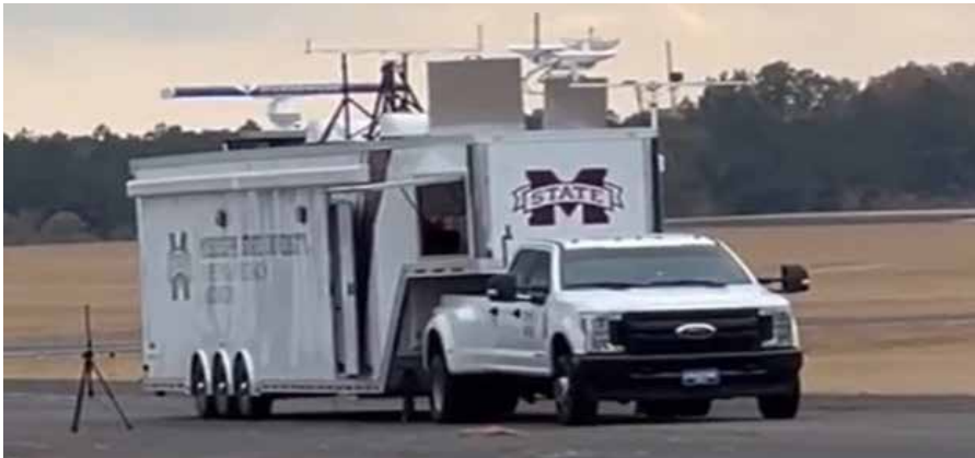
Figure 1. Sparrowhawk marine radar installed on MSU ground control station.
