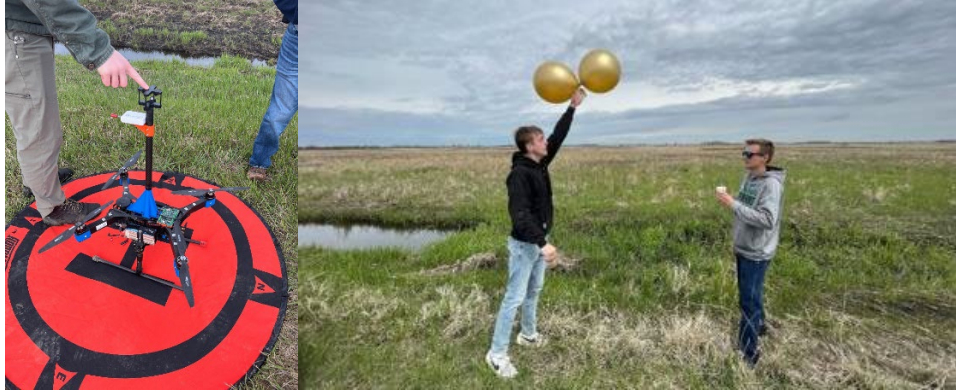
Figure 7. Left: The xFold Spy sUAS integrated with instrumentation including the TriSonica Mini (being pointed at) and an IMET XQ2 (white box with sensor safety cover installed). Right: Students launching a Windsond weather balloon. High visibility balloons were used to improve visibility for the sUAS team.
